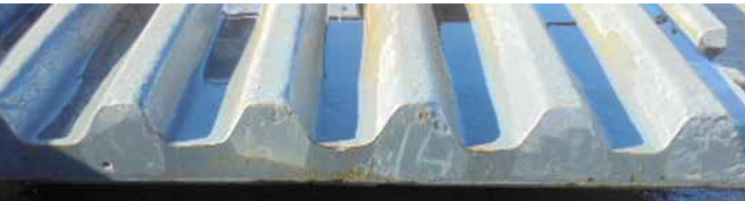
QUARRY SWING JAW – NEW DESIGN – 6 FULL TEETH & 2 HALF TEETH
